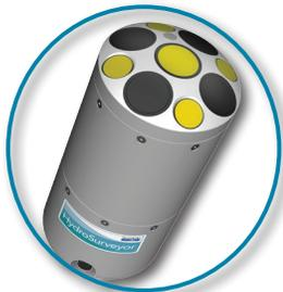
The SonTek **HydroSurveyor-M9** is a system designed to collect bathymetric, water column velocity profile, and acoustic bottom tracking data as part of a hydrographic survey. The two key components of the system are the HydroSurveyor Acoustic Doppler Profiler (ADP®) platform, and the powerful, yet user-friendly, data collection software. Now comes standard with HYPACK and conveniently integrates with the **CastAway®-CTD**.
